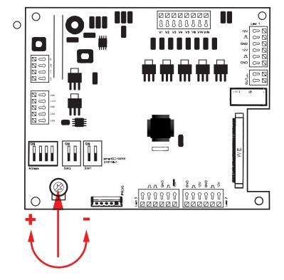
Potentiometer for adjustment of the switch pressure.
