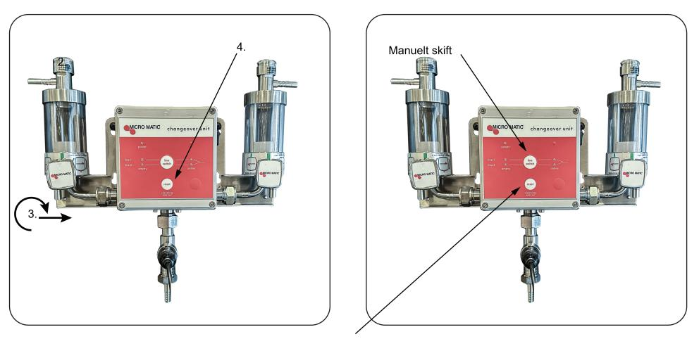
To enter cleaning mode, press the "Reset" -button for more than three seconds.
